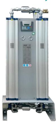
Two towers are filled with adsorbant materials. They are designed to filter H2O molecules by sieving. H2O molecules which adhere to the surface of adsorbent material can be easily separated by the interaction of molecular forces from where they are hold. While the first tower dries the incoming air, the second tower is regenerated with the reverse-direction regenerative air. This is a physical reaction and can be repeated countless times
